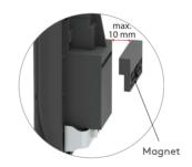
Open-close position of door can be monitored. The max distance between the magnet and the lock is 10 mm.
